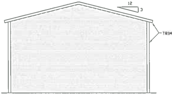
TYPICAL END ELEVATION VERTICAL ROOF SCALE: NTS
